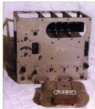
Fig. 5: The Japanese Mk 41 Type D receiver showing the coil pack extracted. The tuning shaft and dial are on the left hand side (see text).
