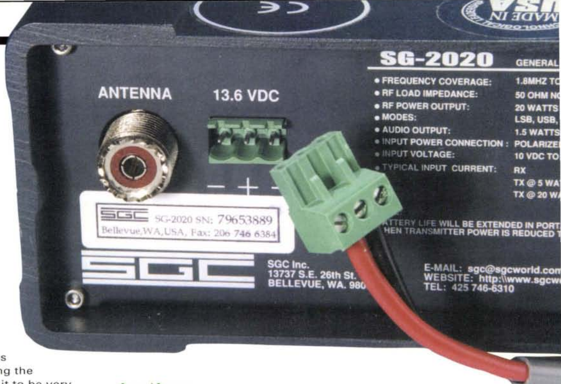
Fig. 4: Rear panel view showing power supply plug and socket (see text for comments). The robustness of the external casing of the transceiver can be judged by the thickness of the casting.
