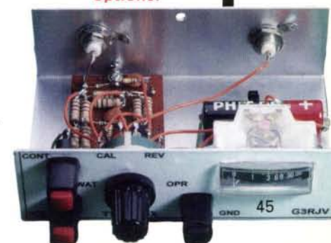
Fig. 5 (Lower): The (very basic) continuity test facilities. See text for G3RJV's notes on expanding this facility to provide individual options.
