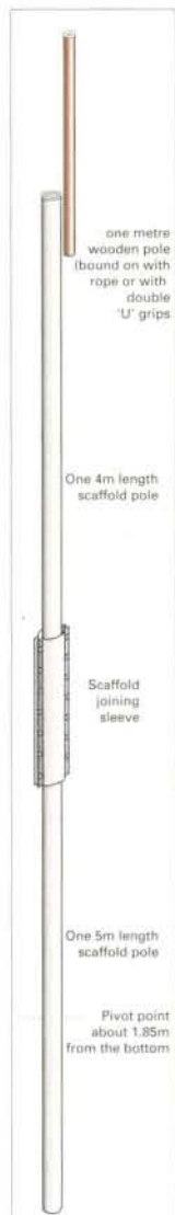
Fig. 1: The 10m length of the mast is achieved by using three lengths joined together.
